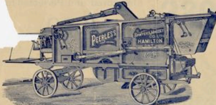
SIDE VIEW OF THE "PEERLESS."—Showing Pulley for Drive Bar and for Beater Belt, and the Guide Pulleys, etc.
