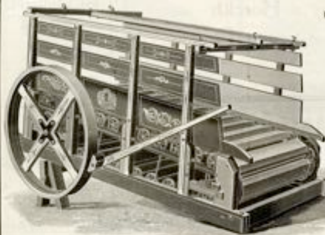
THE NEW "S. & M." LEVEL TREAD POWER, AND JACK.
